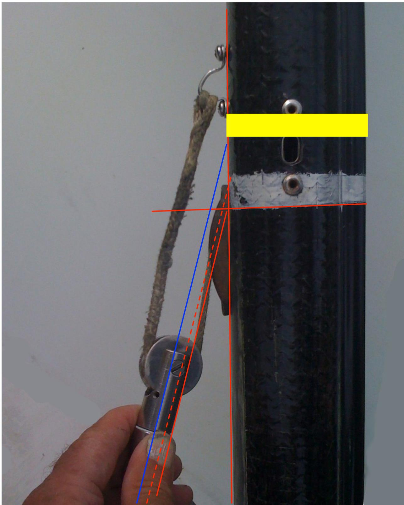
**Figure 5** A 2:1 Genoa halyard system dead ended above the halyard block. The dashed red line shows the 5 mm tolerance and the blue extension of the leading edge of the jib luff wire shows that this rig does not conform to FD class rule 38 by about 6 mm.
