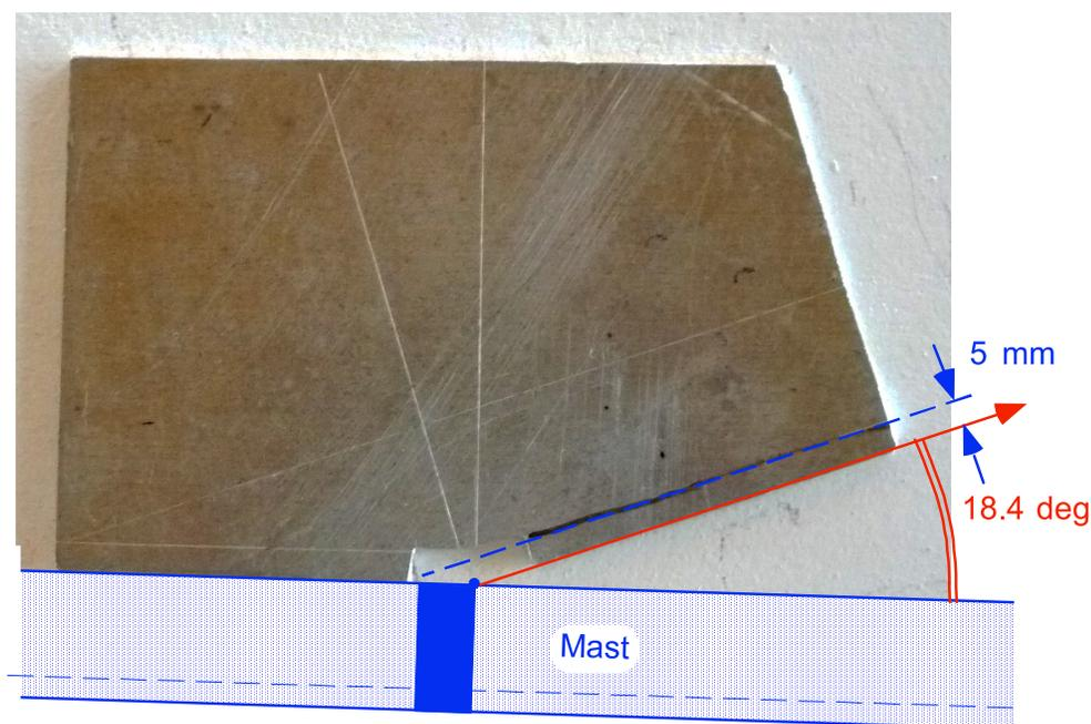
**Figure 3** Jig for determining Genoa luff intersection with front face of the mast. The Genoa halyard is held parallel to the edge (i.e. at  $18.4^{\circ}$  along the red arrow) and no part of the Genoa sail shall be in front of the line on the jig which is at 5 mm from the edge.
