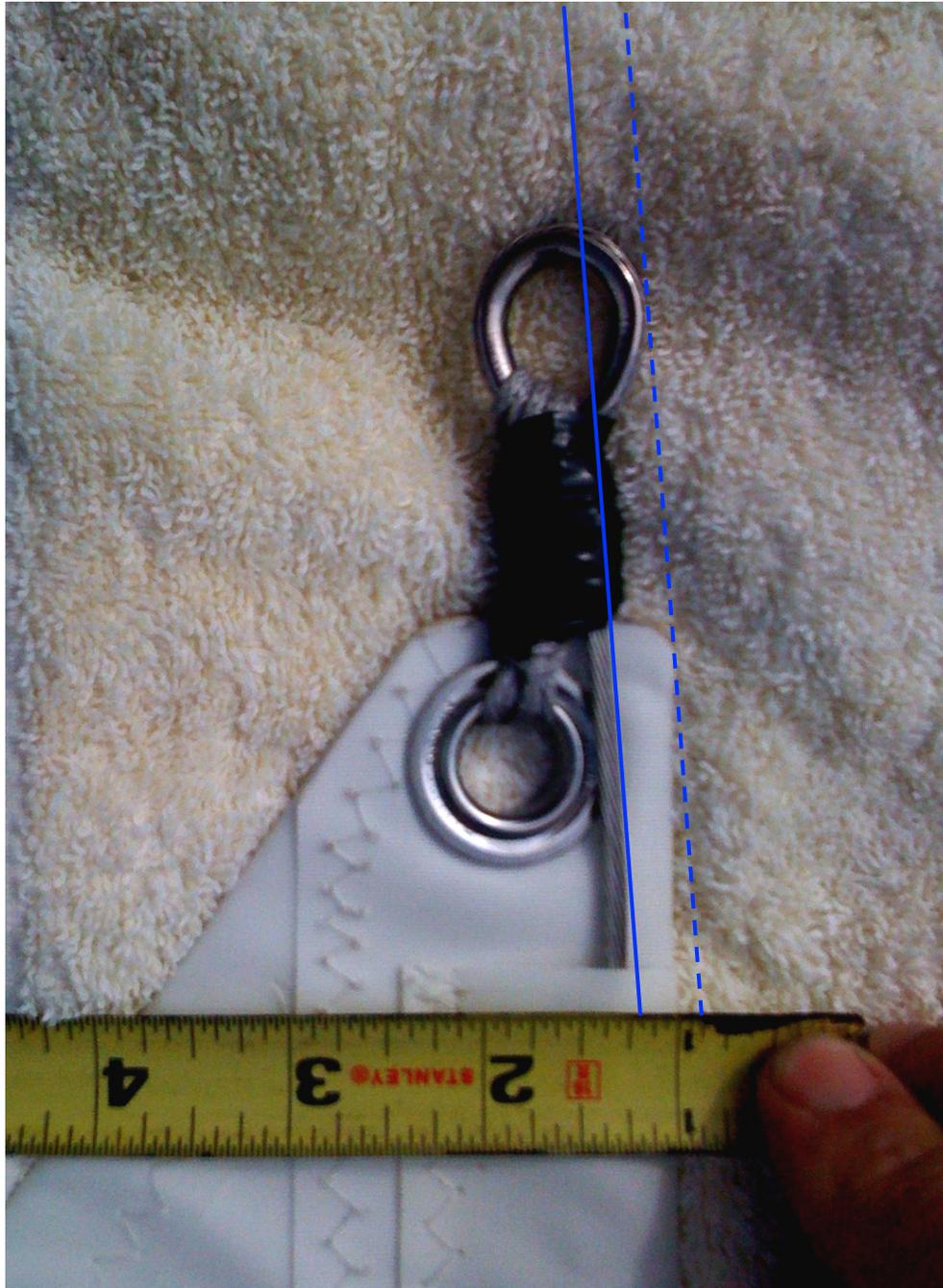
**Figure 4** The head of a North FD Genoa showing that this sail head point extends 8 mm in front of the leading edge of the luff wire.
