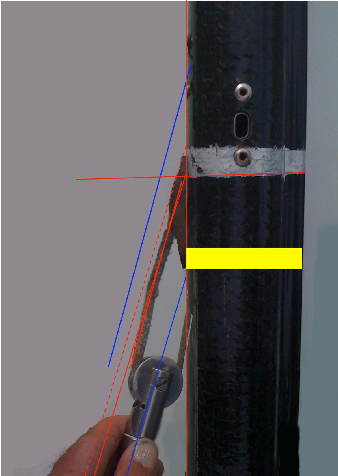
**Figure 6** The same 2:1 Genoa halyard system dead ended below the halyard block. The dashed red line shows the 5 mm tolerance and the blue extension of the leading edge of the jib luff wire shows that this rig easily conforms to FD class rule 38.
